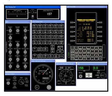
Finally, SSAI develops flight based software applications to increase aircrew situational awareness. The Digital Mapping Interface System (DMIS) provides aircraft and sensor sightline position information via symbology overlaid on a digital moving map. Also included are slant range and DTED based target elevation.
