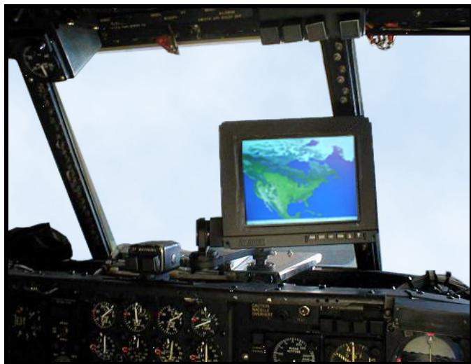
Moving map systems can provide combat aircrews with consolidated information in a format that is tailored to mission needs and is easy to understand at a glance.
